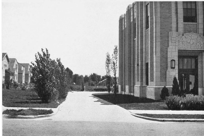
Courtesy of S. Herbert Hare 24d. BUSINESS BUILDING REQUIRED TO HAVE A REAR YARD BECAUSE ABUTTING ON A RESIDENCE DISTRICT, KANSAS CITY, MISSOURI
